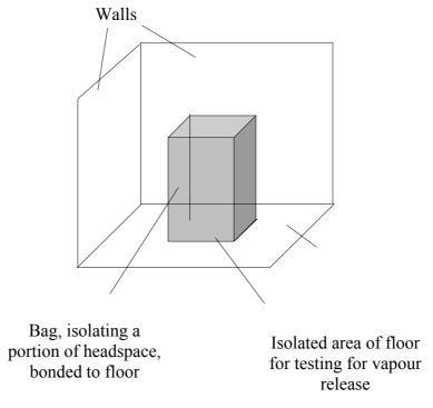
FIGURE 29 METHOD FOR SAMPLING HEADSPACE ABOVE AN ISOLATED AREA OF SOURCE MATERIAL
