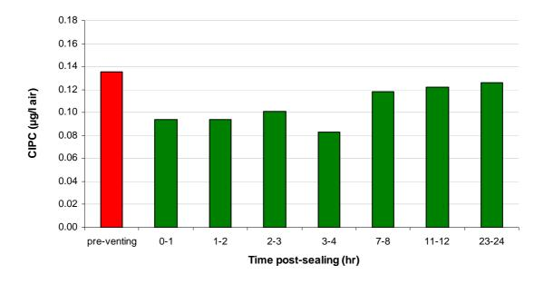
Figure 25 CIPC concentrations in Store 33 in the 24 hours post purging by venting
