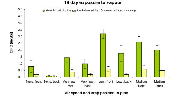
Figure 8 Crop residues in potatoes exposed to CIPC vapour for 19 days before and after 13 weeks efficacy storage at  $10^{\circ}$ C.
