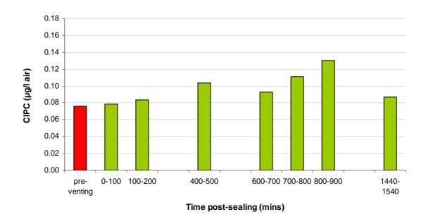
FIGURE 22 CIPC CONCENTRATIONS IN STORE 36 PRE-VENTING AND DURING 24 HOURS POST-VENTING
