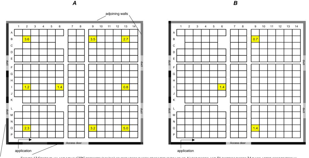
outer walls FIGURE 12 STORE PLAN AND MEAN CIPC DEPOSITS (MG/KG) ON POTATOES TAKEN FROM THE SURFACE OF A) TOP BOXES AND B) BOTTOM BOXES 24 DAYS AFTER CONVENTIONAL APPLICATION (SINGLE PORT)
