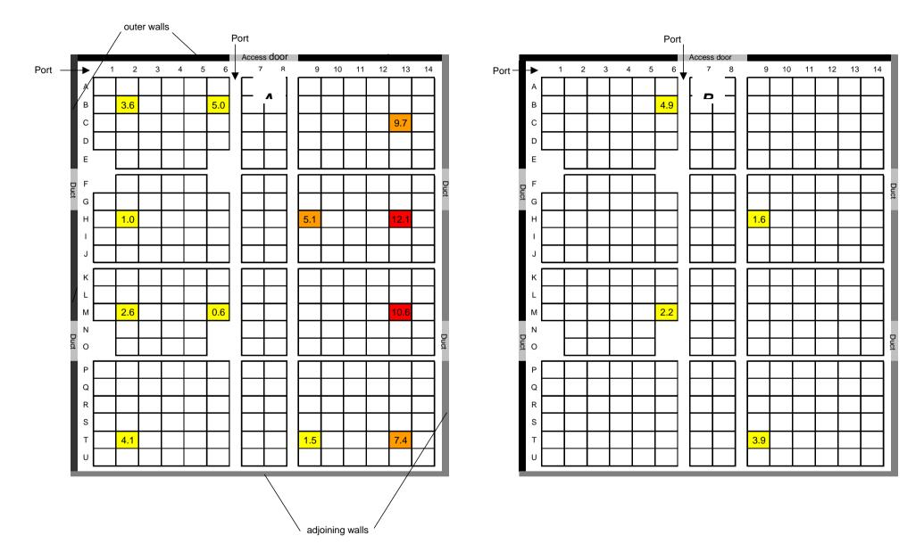
FIGURE 11 MEAN CIPC DEPOSITS (MG/KG) ON POTATOES TAKEN FROM THE SURFACE OF A) TOP BOXES AND B) BOTTOM BOXES 24 DAYS AFTER MULTI-PORT APPLICATION
