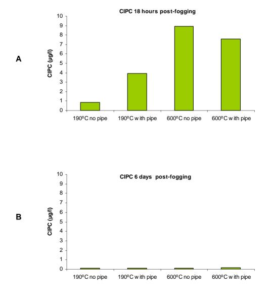
FIGURE 11: CIPC CONCENTRATIONS IN AIR SAMPLES COLLECTED ON TENAX A) 18 HOURS AND B) 6 DAYS POST-APPLICATION. NOTE THAT GRAPHS ARE ON THE SAME SCALE.
