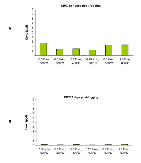
FIGURE 14: CIPC CONCENTRATIONS IN SAMPLES COLLECTED ON TENAX A) 18 HOURS AND B) 7 DAYS POST-APPLICATION.
