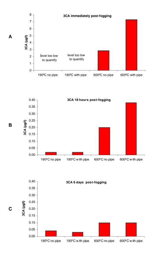
Figure 10: 3-chloroaniline concentrations in samples collected on Tenax A) immediately B) at 18 hours and C) 6 days post-application
